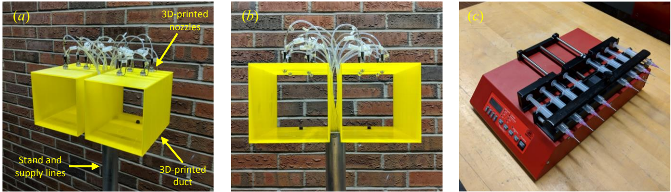
Fig. 2 Components of the full-scale system. (a) Annotated photograph of the two-module HFSB generator. (b) Front view of the HFSB generator; each module has dimensions 20 \times 15 \times 15 \text{ cm}^3 . (c) The multi-syringe pump used to regulate BFS to each of the 8 nozzles.
