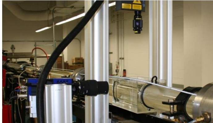
FIG 3. The PIV/PTV setup consists of a camera imaging perpendicular to the laser sheet. The test section of the flow loop is contained in a glycerol box minimizing distortion effects caused by the round glass pipe.
